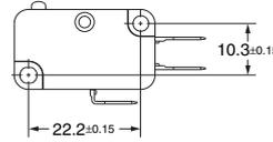
Note. Switches with the mounting holes shown in the diagram can be used except for special models.
